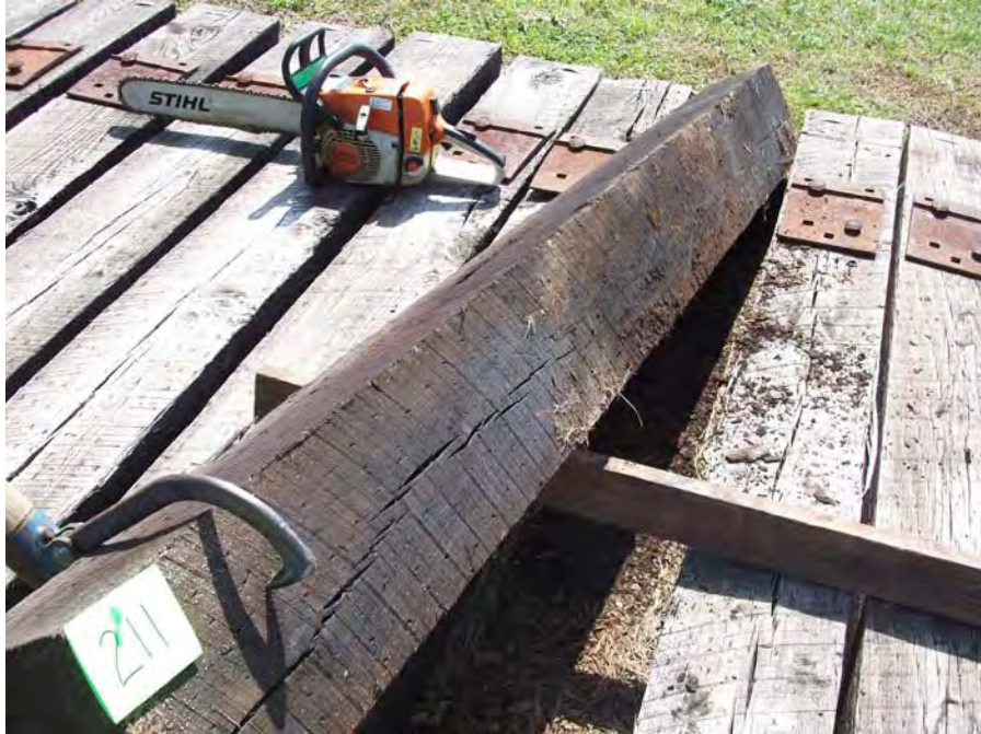
Figure 97 – Tie #211 red oak/borate/creosote 7lbs (Koppers).
