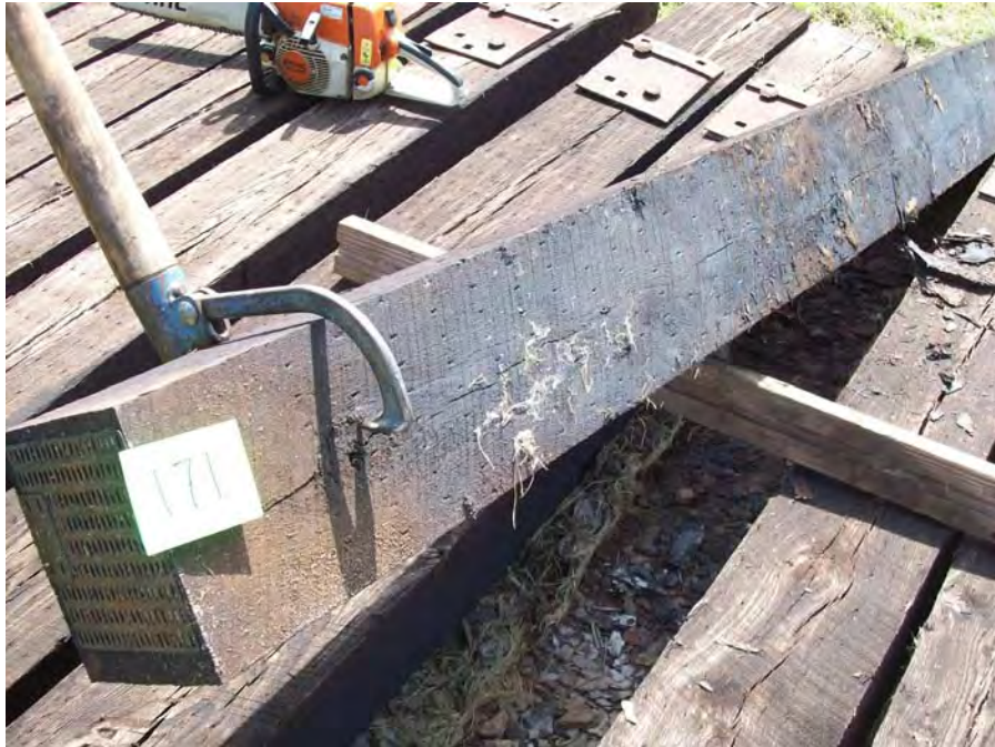
Figure 89 – Tie #171 white oak/DOT/ACZA/oil (Lonza).
