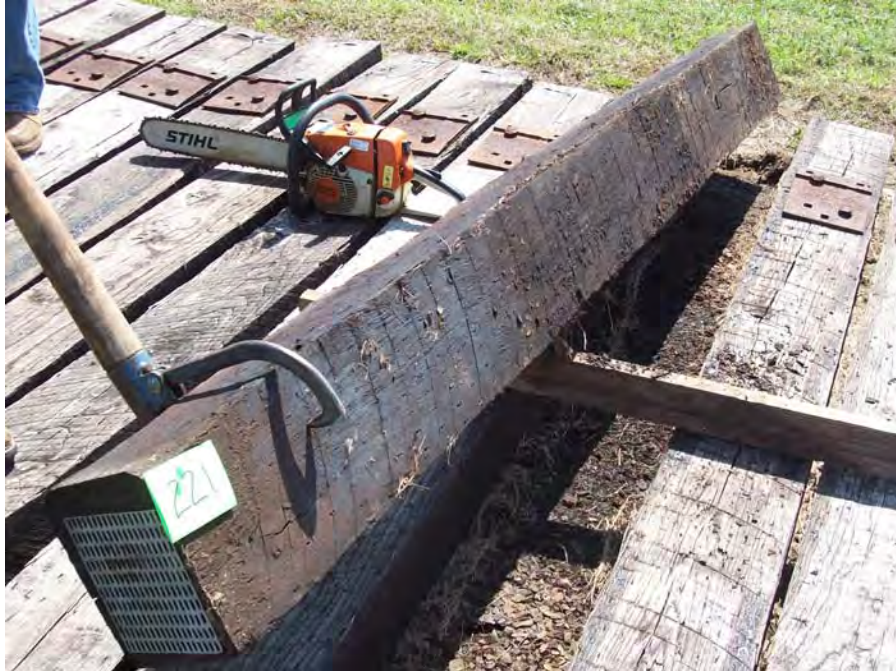
Figure 99 – Tie #221 red oak/borate/creosote 6lbs (Koppers).
