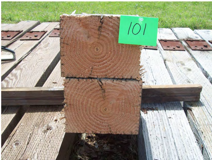
Figure 74 - Tie #101 untreated Douglas fir.
