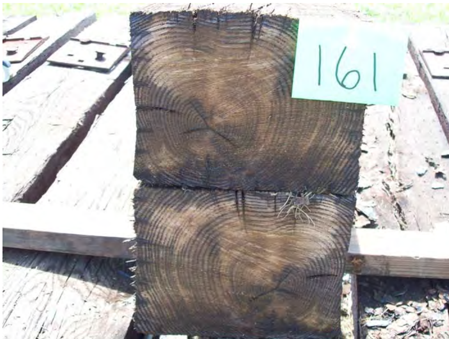
Figure 88 - Tie #161 red oak/DOT/ACZA/oil (Lonza).
