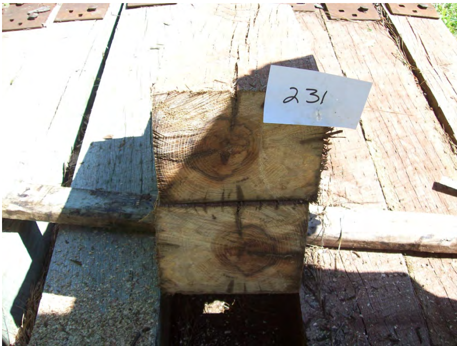
Figure 50 - Tie # 231 white oak/DOT/ACZA/ET (Lonza).
