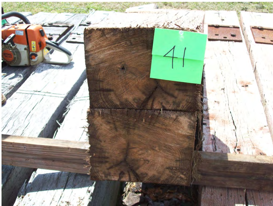
Figure 62 - Tie #41 white oak/DOT/ACZA/ET (Lonza).
