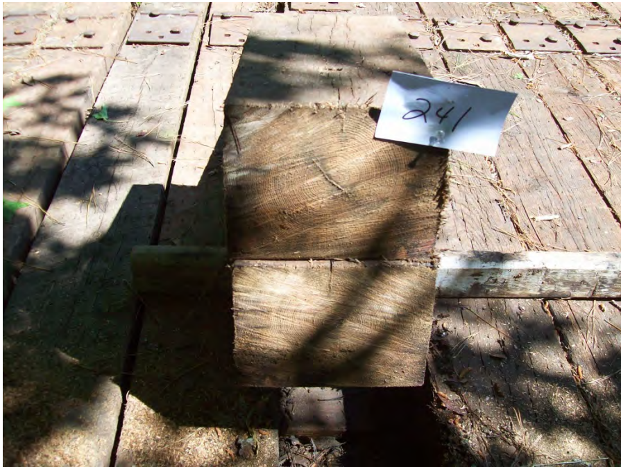
Figure 52 - Tie #241 red oak/ACZA/DOT/ET (Lonza).
