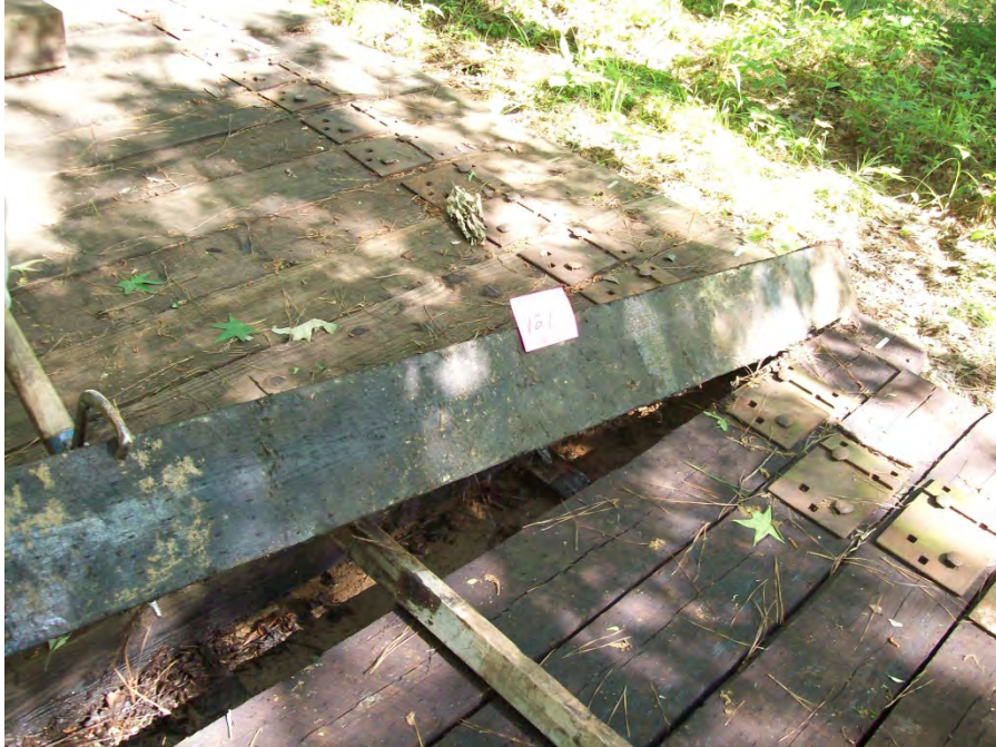
Figure 25 – Tie #121 red oak/DOT/ACZA/oil (Lonza).
