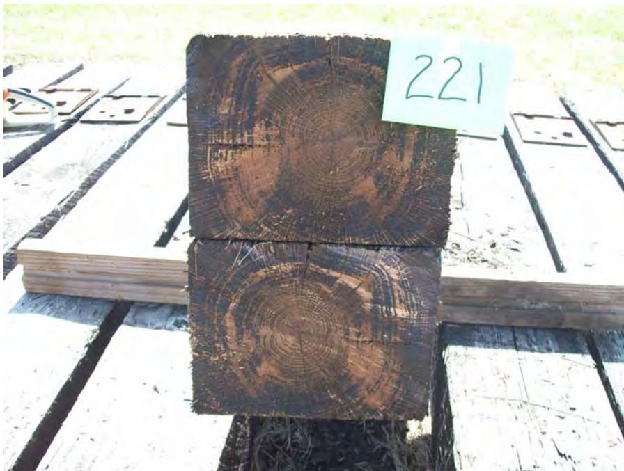
Figure 100 - Tie #221 red oak/borate/creosote 6lbs (Koppers).
