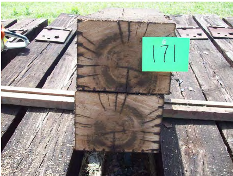
Figure 90 – Tie #171 white oak/DOT/ACZA/oil (Lonza).
