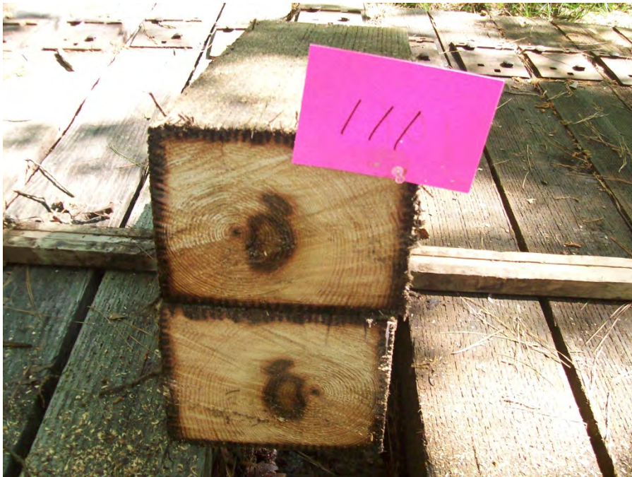
Figure 24 - Tie #111 Douglas fir/DOT/ACZA (Lonza).
