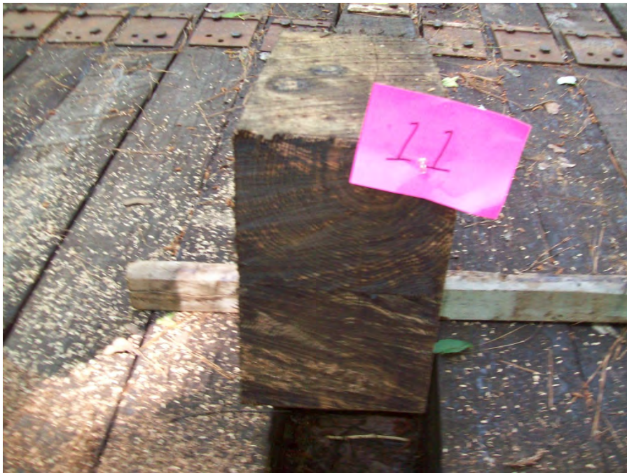
Figure 4 - Tie #11 red oak/borate/creosote 7lbs (Koppers).
