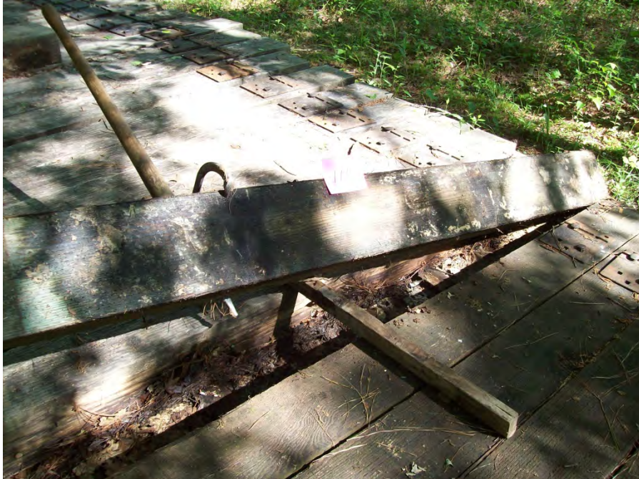
Figure 23 – Tie #111 Douglas fir/DOT/ACZA (Lonza).
