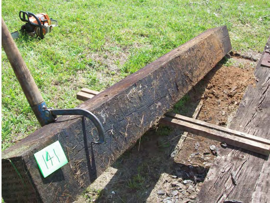
Figure 81 – Tie #141 red oak/DOT/ACZA/oil (Lonza).
