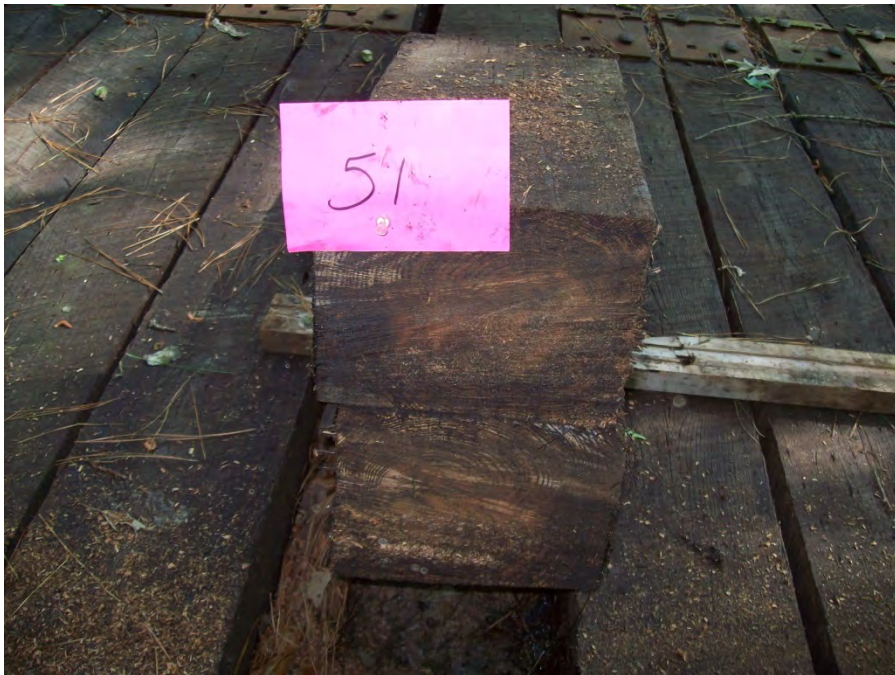
Figure 12 - Tie #51 red oak/borate/creosote 6lbs (Koppers).
