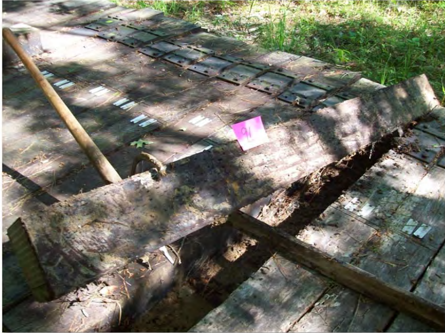
Figure 19 – Tie # 91 untreated white oak.
