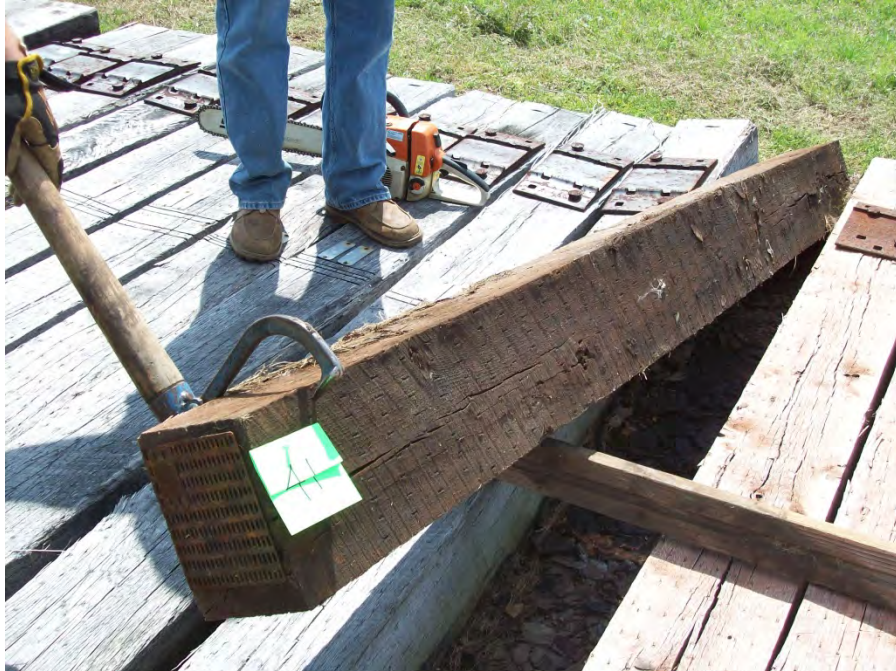
Figure 61 – Tie #41 white oak/DOT/ACZA/ET (Lonza).
