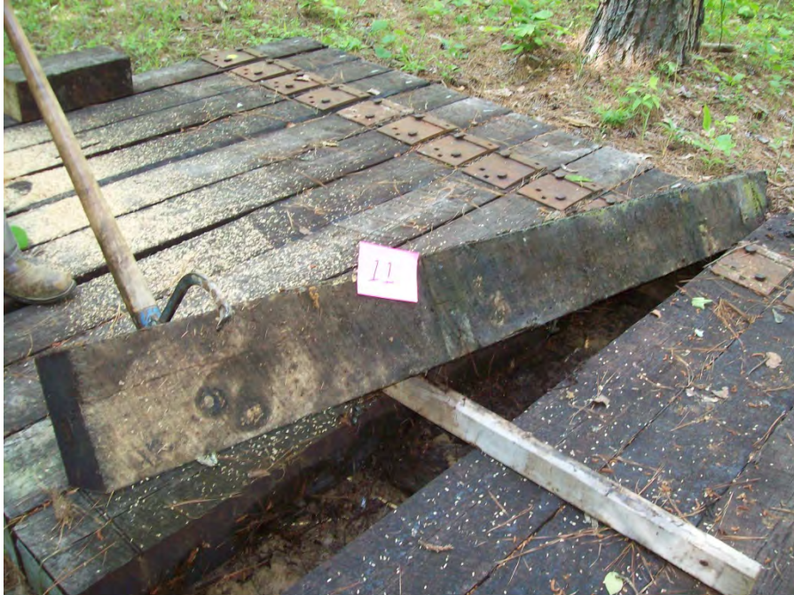
Figure 3 - Tie #11 red oak/borate/creosote 7lbs (Koppers).
