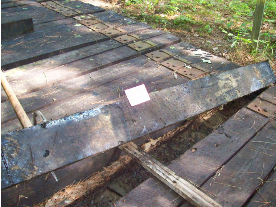
Figure 11 - Tie #51 red oak/borate/creosote 6lbs (Koppers).
