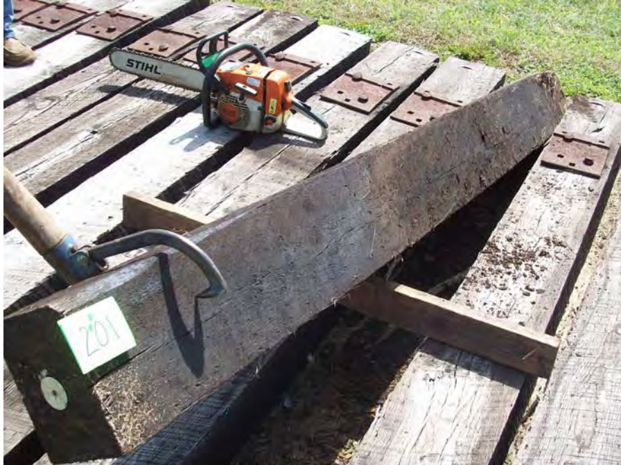
Figure 95 – Tie #201 white oak/borate/creosote 7lbs (Koppers).
