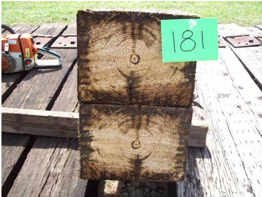
Figure 92 - Tie #181 Douglas fir/P2 (Lonza).
