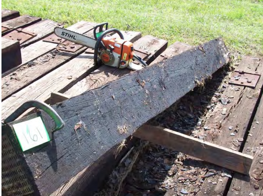
Figure 87 – Tie #161 red oak/DOT/ACZA/oil (Lonza).
