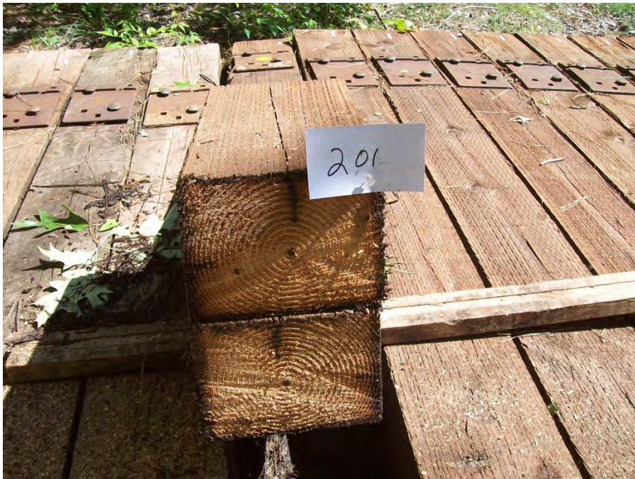
Figure 44 - Tie #201 Douglas fir/ACZA/DOT/ET (Lonza).
