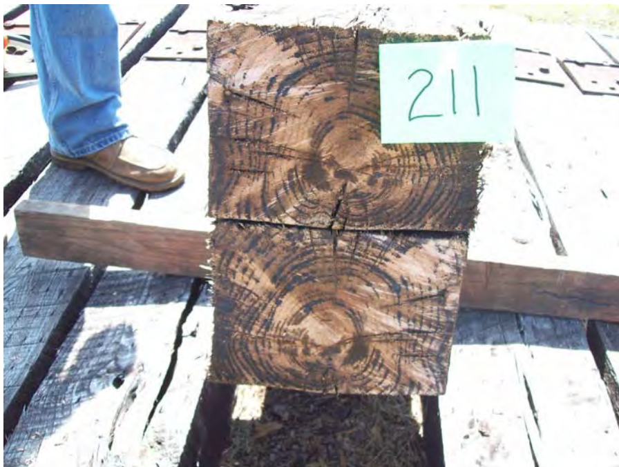
Figure 98 - Tie #211 red oak/borate/creosote 7lbs (Koppers).
