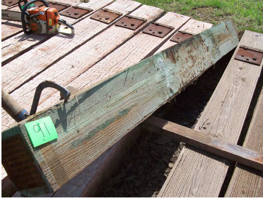
Figure 71 – Tie #91 Douglas fir/DOT/ACZA (Lonza).
