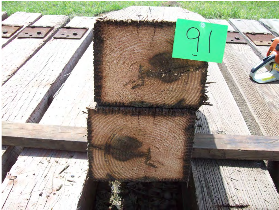
Figure 72 - Tie #91 Douglas fir/DOT/ACZA (Lonza).
