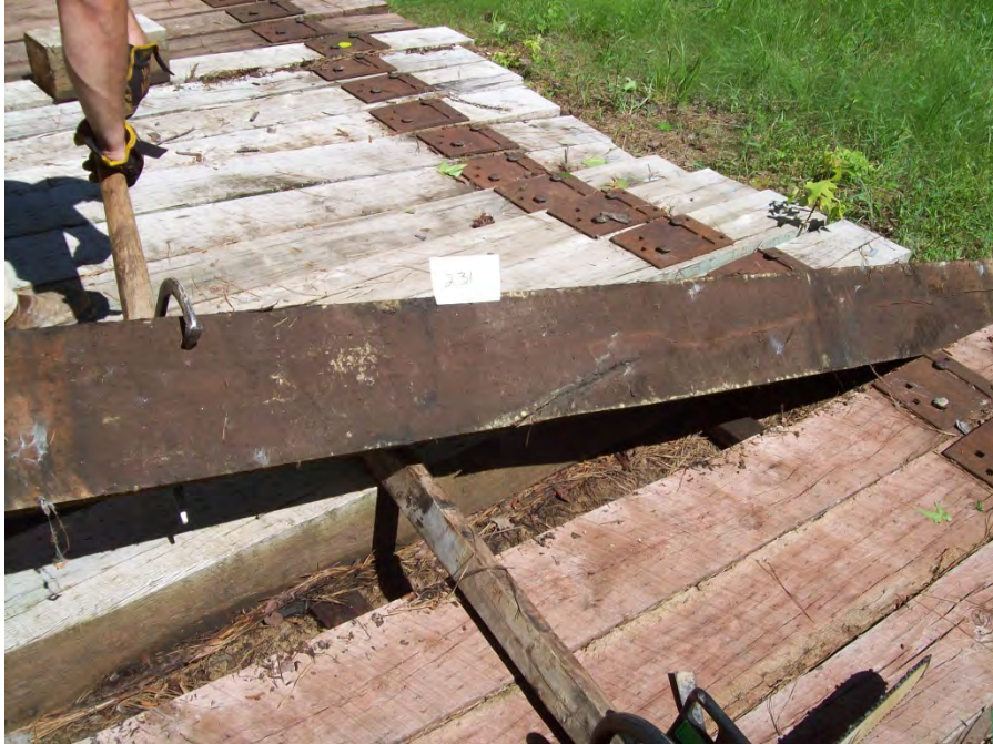
Figure 49 – Tie # 231 white oak/DOT/ACZA/ET (Lonza).
