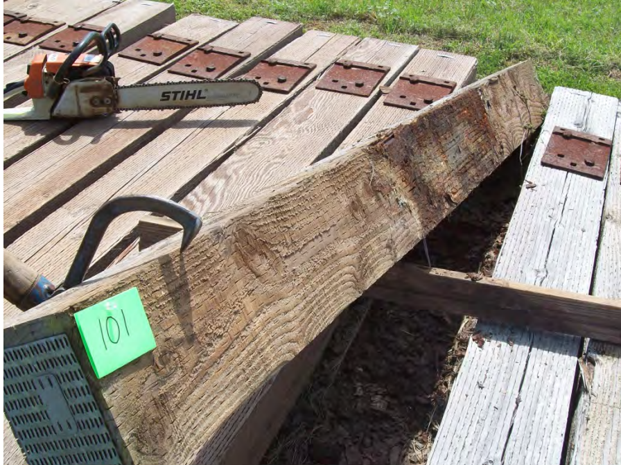
Figure 73 – Tie #101 untreated Douglas fir.
