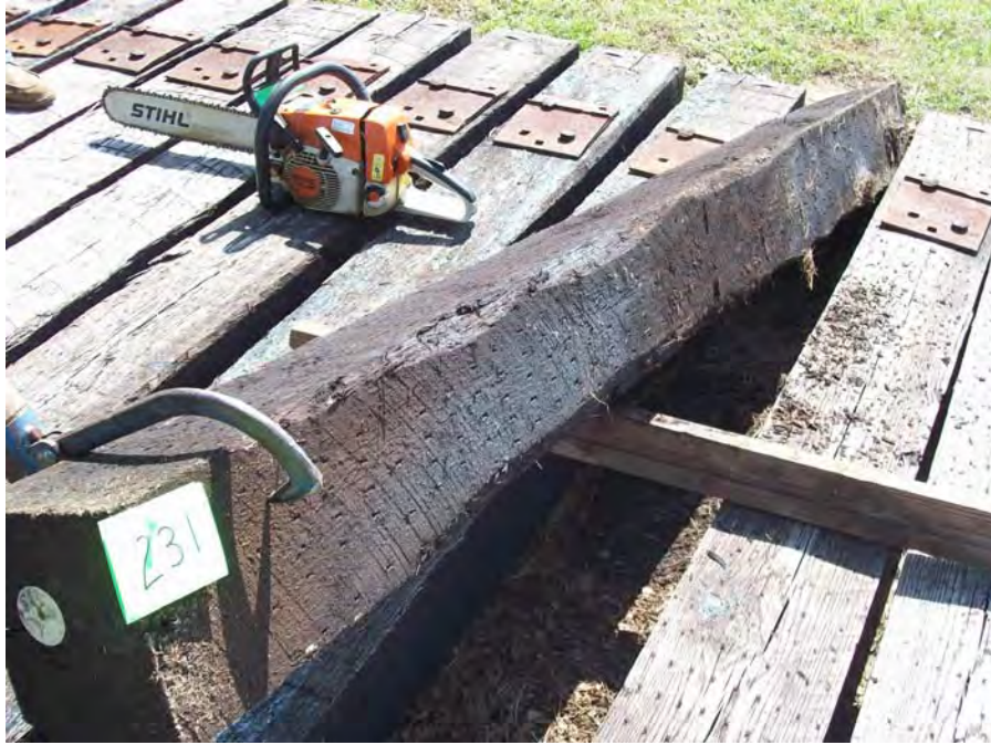
Figure 101 – Tie #231 red oak/creosote 7lbs (Koppers).
