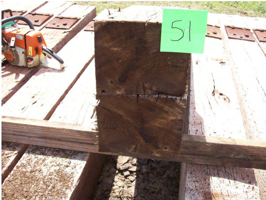
Figure 64 - Tie #51 red oak/DOT/ACZA/ET (Lonza).
