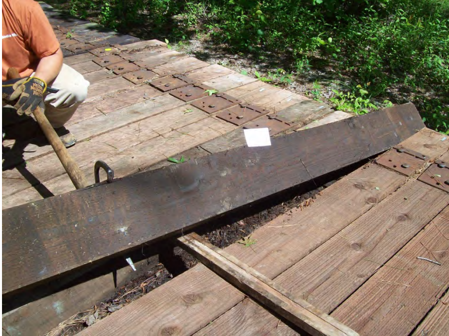
Figure 43 – Tie #201 Douglas fir/ACZA/DOT/ET (Lonza).
