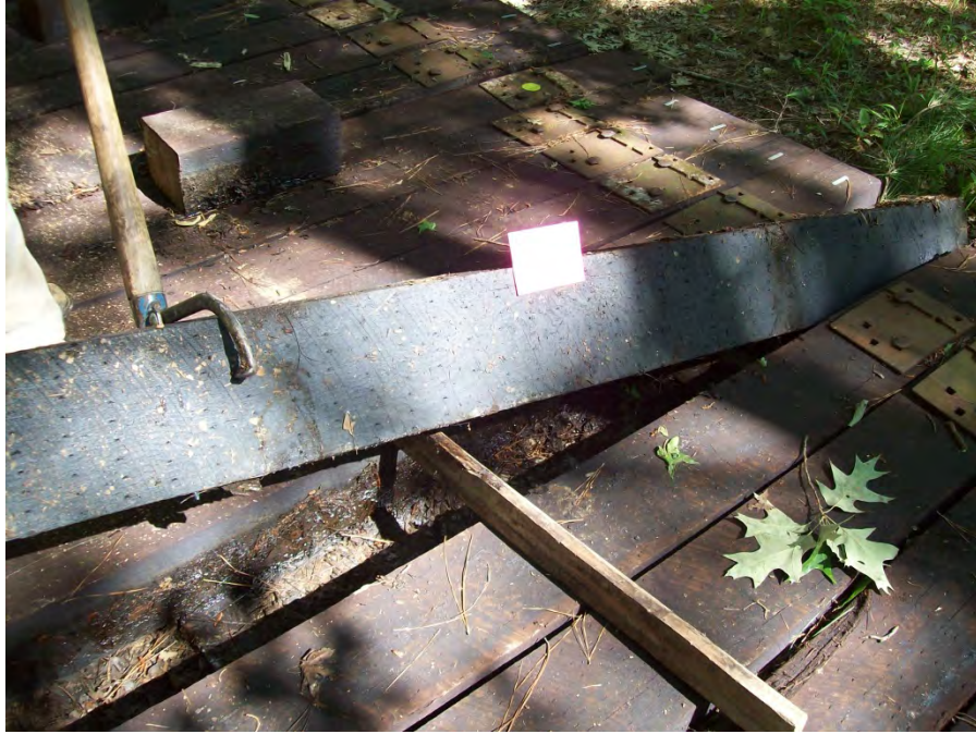
Figure 31 – Tie #141 white oak/DOT/ACZA/oil (Lonza).
