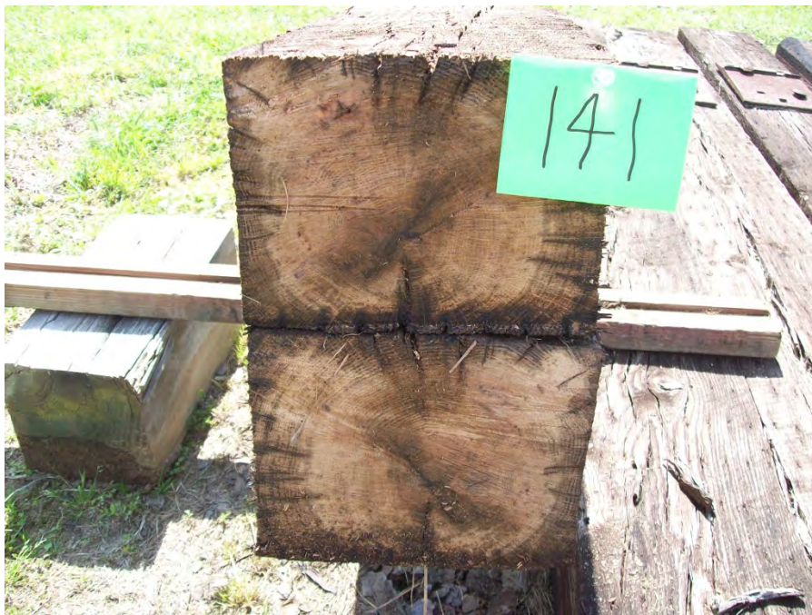
Figure 82 – Tie #141 red oak/DOT/ACZA/oil (Lonza).
