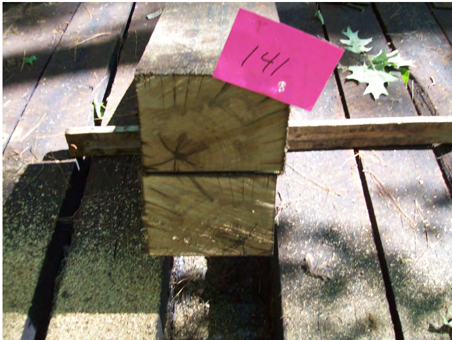
Figure 32 - Tie #141 white oak/DOT/ACZA/oil (Lonza).
