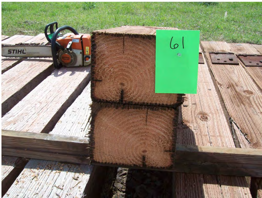
Figure 66 - Tie #61 Douglas fir/DOT/ACZA/ET (Lonza).
