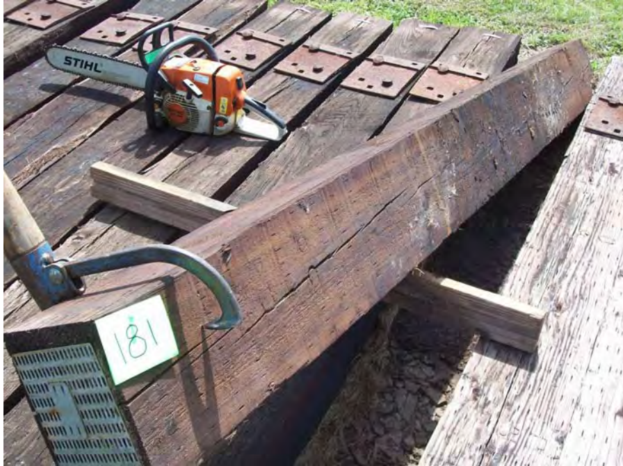
Figure 91 – Tie #181 Douglas fir/P2 (Lonza).
