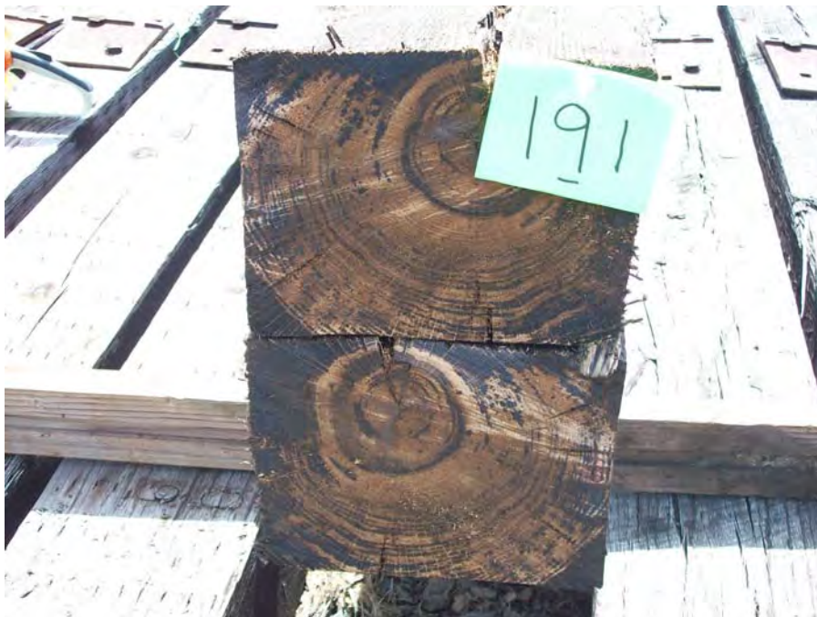
Figure 94 - Tie #191 white oak/borate/creosote 6lbs (Koppers).
