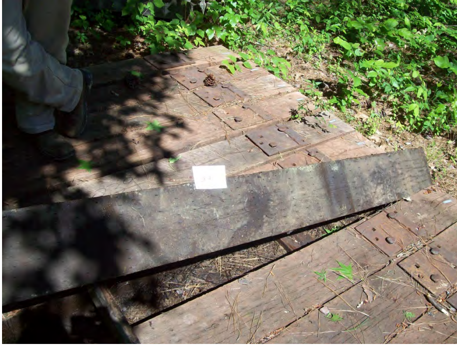
Figure 51 – Tie #241 red oak/ACZA/DOT/ET (Lonza).
