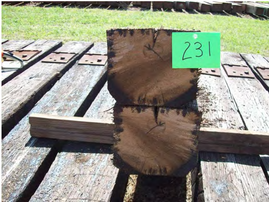
Figure 102 - Tie #231 red oak/creosote 7lbs (Koppers).
