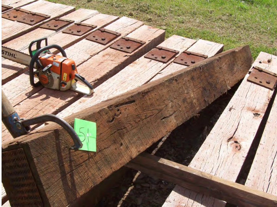
Figure 63 – Tie #51 red oak/DOT/ACZA/ET (Lonza).
