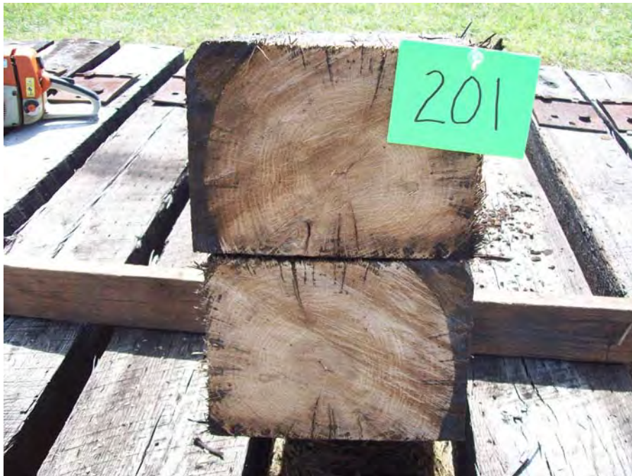
Figure 96 - Tie #201 white oak/borate/creosote 7lbs (Koppers).
