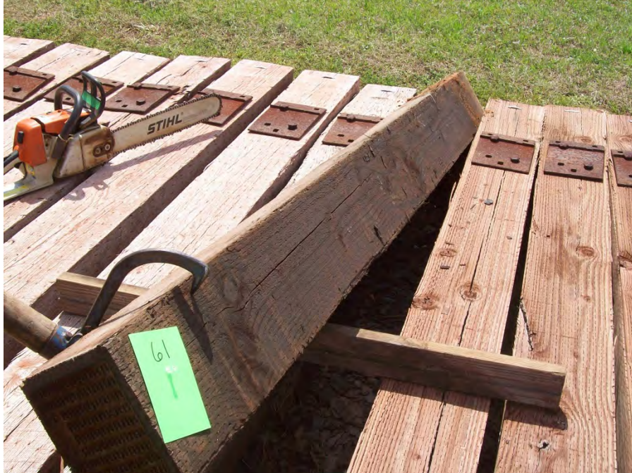
Figure 65 – Tie #61 Douglas fir/DOT/ACZA/ET (Lonza).
